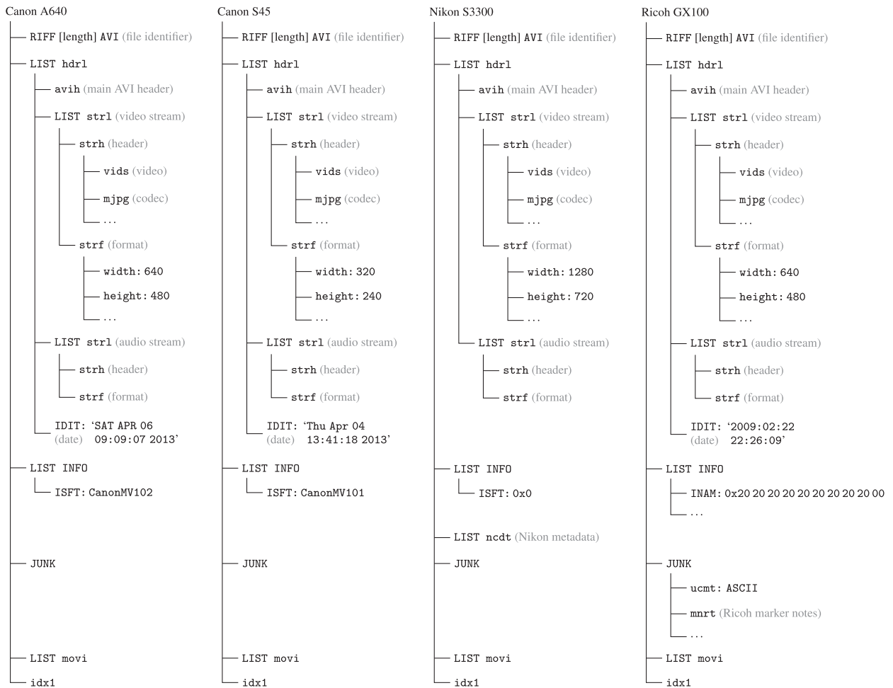
Fig. 2. AVI file structure of videos acquired with Canon A640, Canon S45, Nikon CoolPixS3300, and Ricoh GX100 digital cameras. Equivalent elements are arranged on the same horizontal level. Not all nested sub-elements are listed.
