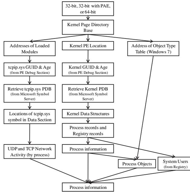
Fig. 1 – A Windows-agnostic memory analysis process flow.
