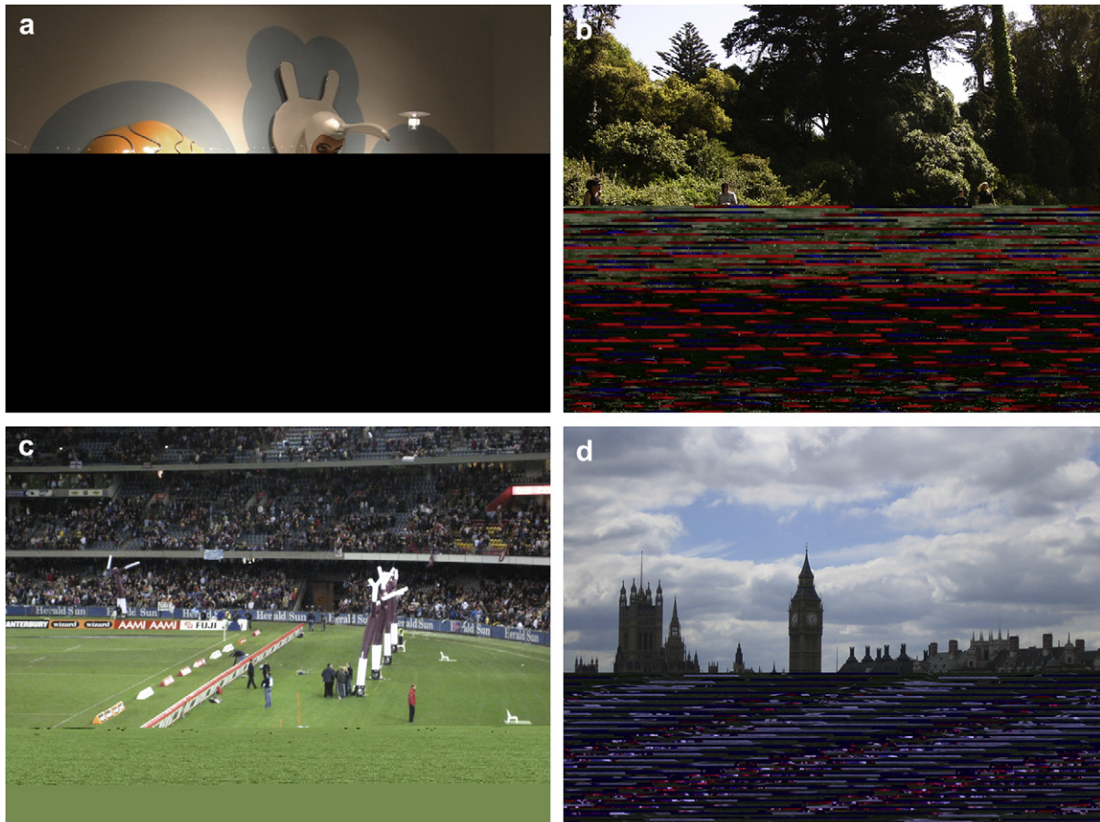
Fig. 5 – Four images from the DFRWS 2007 test-set that are decoded incorrectly when doing sequential decoding.
