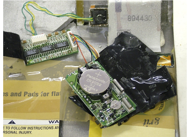
Fig. 4 – Components from a Mini-123 used in an imitation ATM fascia.
