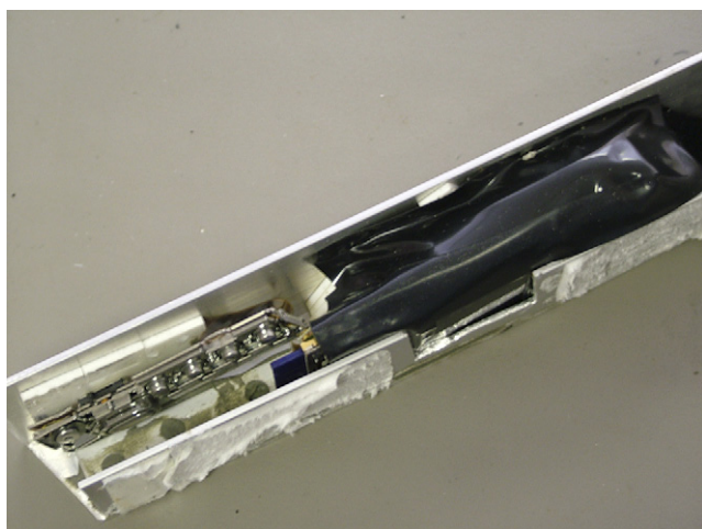
Fig. 7 – Rear view of plastic strip showing the components of a small digital camera.
