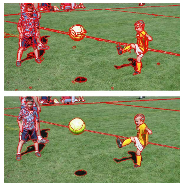
Fig. 2 – Results of mean-shift segmentation with parameters h_s = 7 , h_r = 6 , and M = 50 (top). Results of region merging (bottom).
